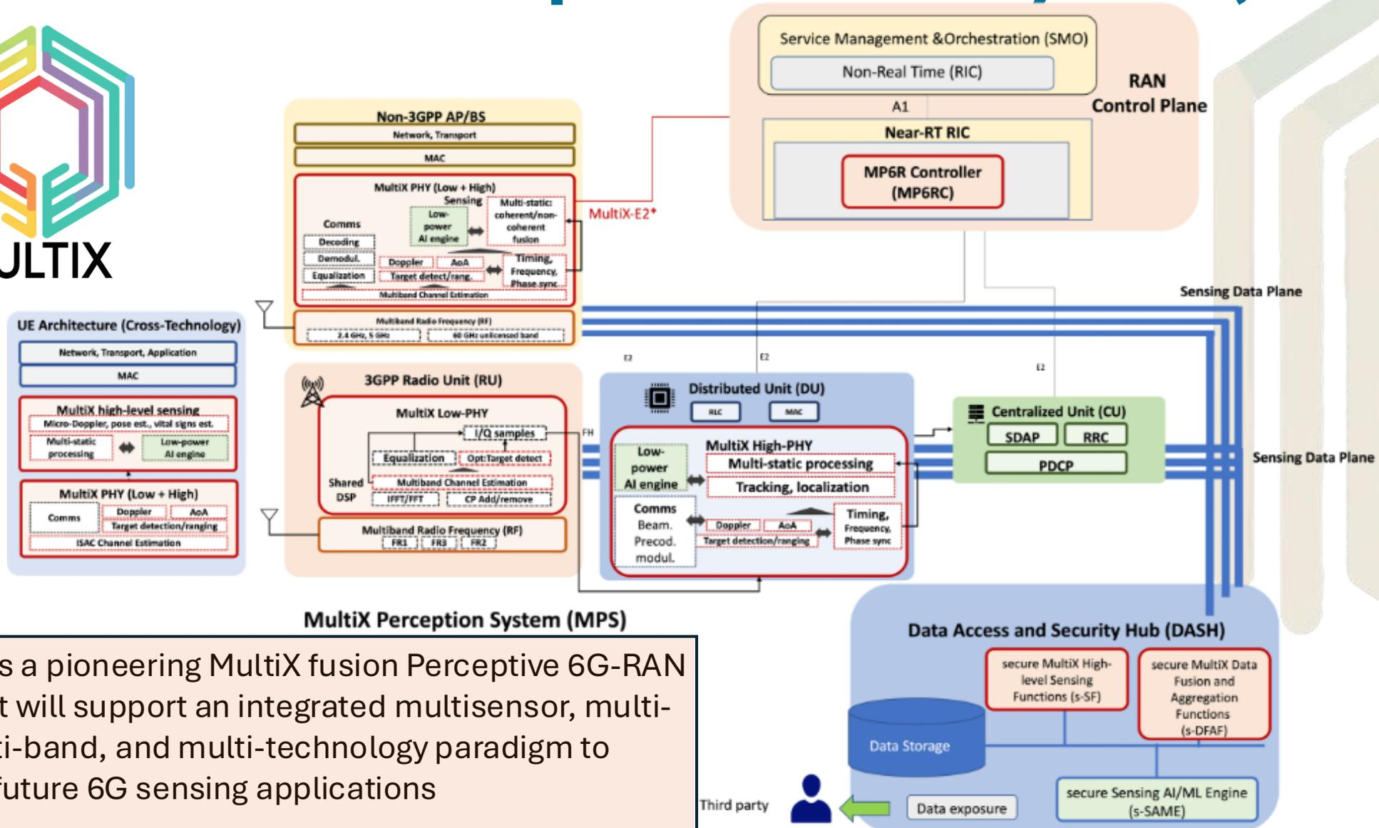
The MP6R is a pioneering MultiX fusion Perceptive 6G-RAN system that will support an integrated multisensor, multi-static, multi-band, and multi-technology paradigm to enable for future 6G sensing applications
