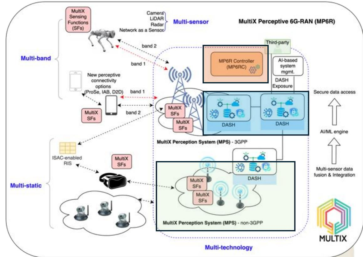
**Data Access and Security Hub (DASH)** designed as a novel RAN data plane entity that aggregates multi-sensor data of diverse technologies, providing secure data access, processing, storage, and exposure, ensuring data privacy and trustworthiness, and that can be fully distributed throughout the data plane wherever needed in the 6G-RAN.
