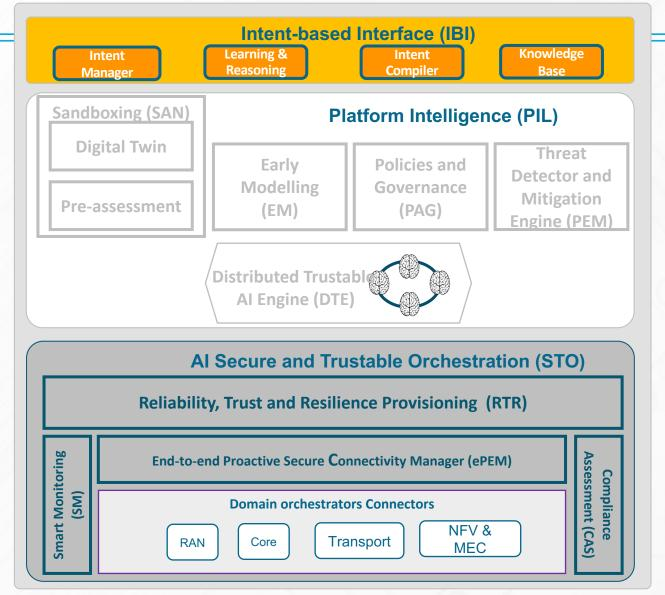
The Intent-Based Interface (IBI) is responsible for mapping high-level intents into security workflows able to react to security threats and vulnerabilities, which will itself use AI for intent optimisation:
